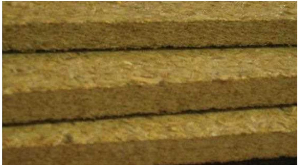
*Particle boards from wood chips or sawdust needs binder. The synthetic binder are usually formaldehyde that emits dangerous substance dangerous for environment and our health.*
